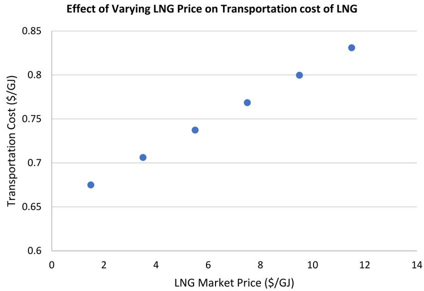
Fig. 4. Sensitivity analysis on transportation cost of LNG as market price of LNG is varying from (1.5 to 12 \$/GJ).
