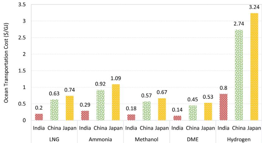
Fig. 8. Costs for transporting natural gas energy via various energy carriers from Qatar to India, China, and Japan.
