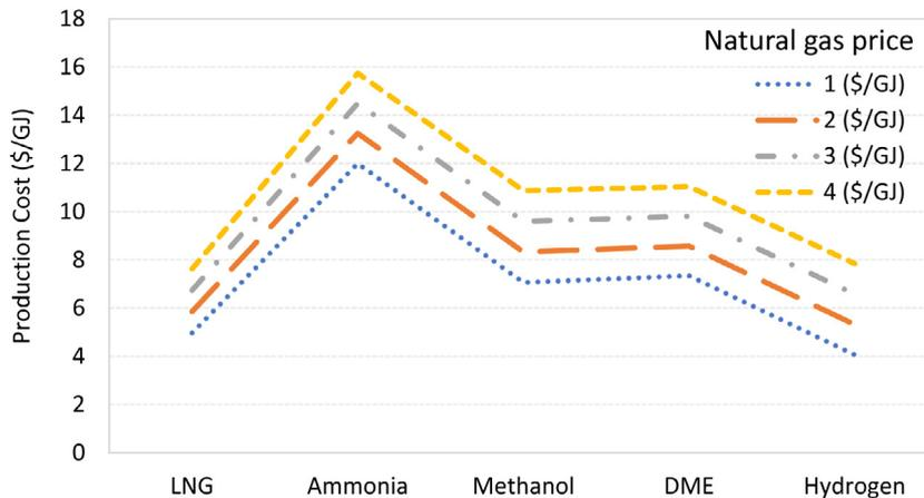
Fig. 3. Effects of changing the cost of natural gas on the total production cost of energy carriers.
