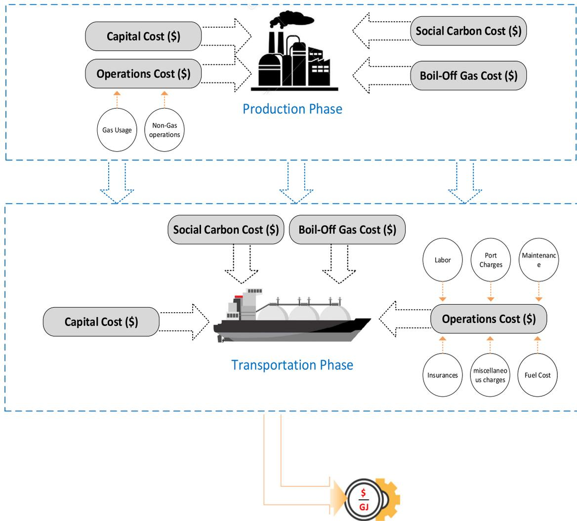
Fig. 1. The involved phases to determine the total cost of a liquefied energy carrier.
