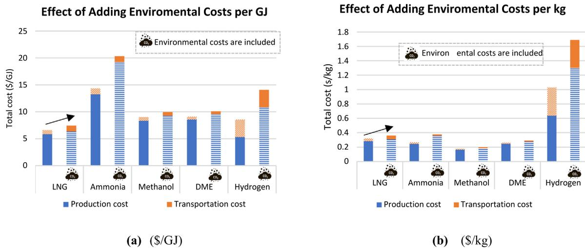
Fig. 9. Effect of adding environmental cost (0.137 \$/kg CO<sub>2</sub> eq.) within the total cost of various energy carriers per (a) GJ and (b) per kg.
