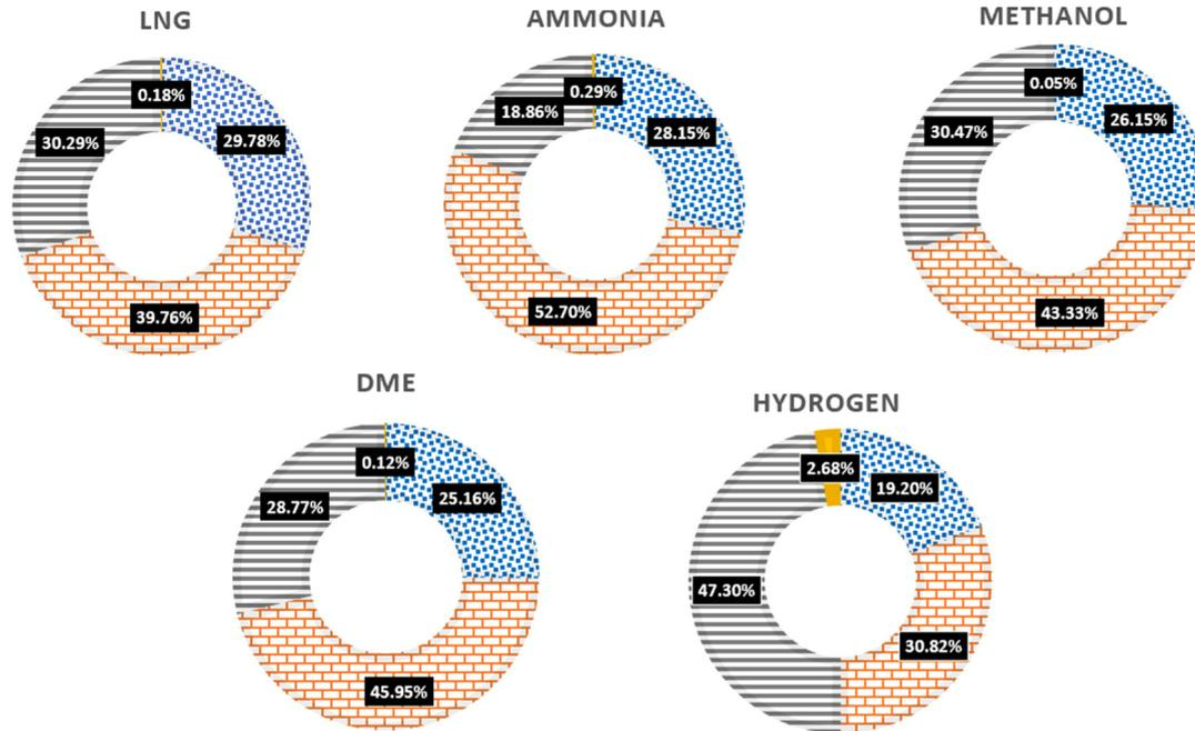
Fig. 2. Cost breakdown of producing various energy carriers.
