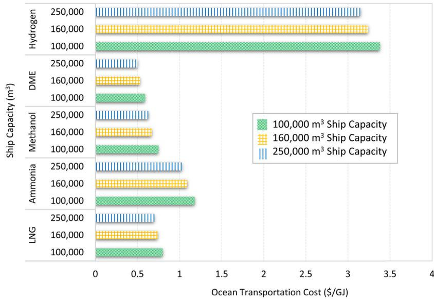
Fig. 7. Sensitivity analysis on ocean transportation cost for various energy carriers based on ship capacity.
